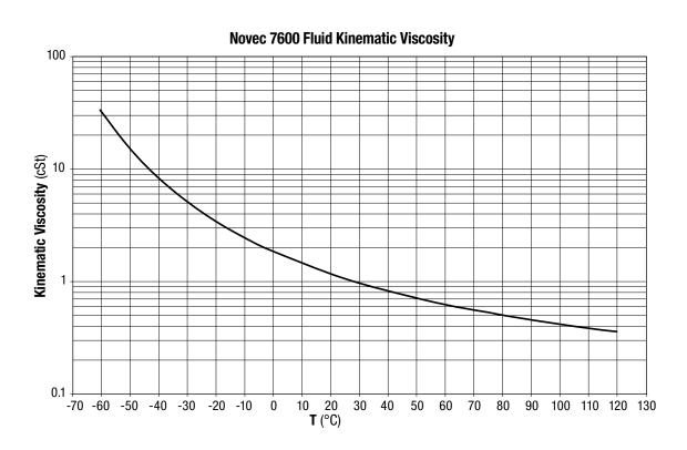
Kinematic Viscosity, centistokes = EXP ( $464.403382/(T[^{\circ}C]+133)-2.881482$
